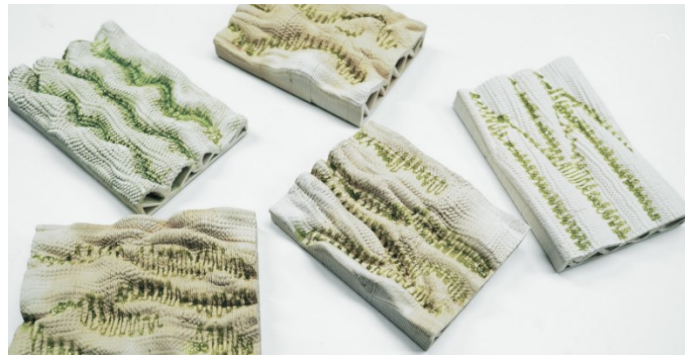
Figure 7. 3D Printed Algae Panels showcasing an innovative approach to bio-integrated architectural design that supports biodiverse sustainability (by The Bio integrated lab UCL, 2023)
