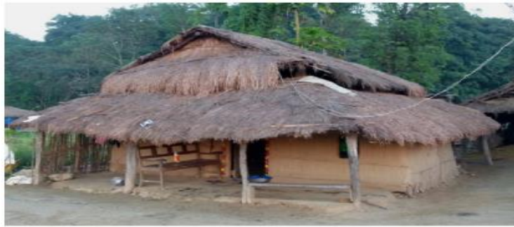
Figure 3. Tharu house with wide roof overhang and shaded veranda in Chitwan (Bodach, & Hamhaber, 2014).
